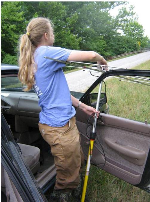
Figure 3 – a 5 element Yagi mounted on a painter's pole use through the window of a car
