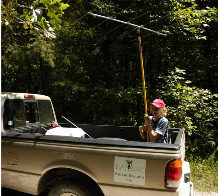
Figure 2 – a 5 element Yagi mounted on a painter's pole used in the bed of a pickup truck
