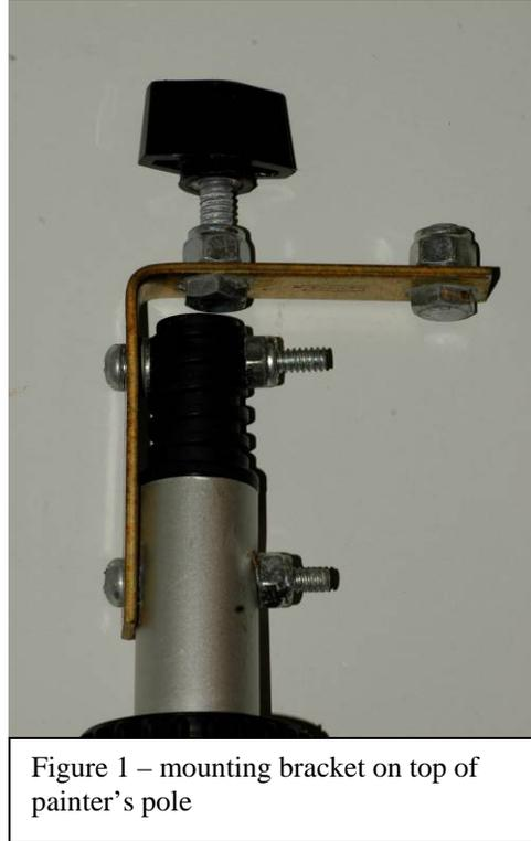
Figure 1 – mounting bracket on top of painter's pole
